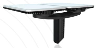
The Hughes HL1120W User Terminal (UT) includes a low-profile Electronically Steered Antenna (ESA) that represents the leading edge of Low Earth Orbit (LEO) antenna technology. The HL1120W ESA is a full-duplex, self-aligning terminal with a built-in modem. It has no moving parts and is optimized for operation over the OneWeb Ku-band LEO satellite constellation – providing access to affordable, fast, high bandwidth and low latency communications service.
